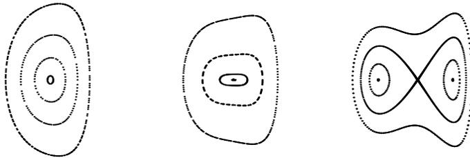
Figure 5: Period-doubling bifurcation in an area-preserving mapping.
